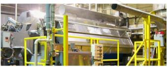
All of our reactors are agitated, steamheated, and water-cooled, served by dual liquid-ring vacuum systems; three reactors have over-head condensers and two of those have internal cooling/heating coils.
